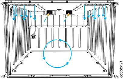
Fig. 4 Schematic view of the internal airflow
