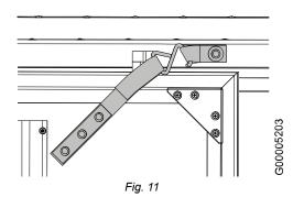
**2.** Steer the container on the roller bed system using the straps on the outside corners.
