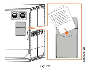
15. Optional: Seal the control unit with a security seal inserted through the slot in the latch. For security seal properties, refer to 3.4 Attachment points for security seals.
