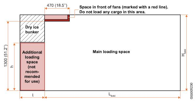
Fig. 48 Loading space, side view
