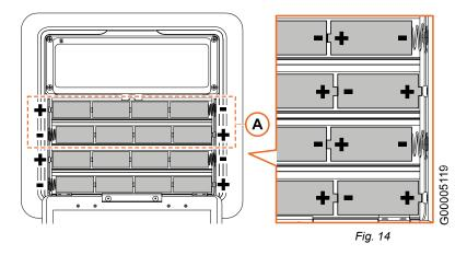
**2.** Place 16 D-cell alkaline batteries in the holder, ensuring proper battery polarity. Battery characteristics:
