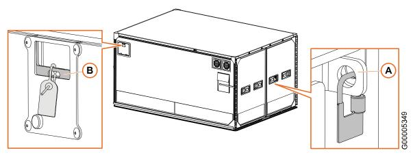
Fig. 5 Attachment points for security seals
